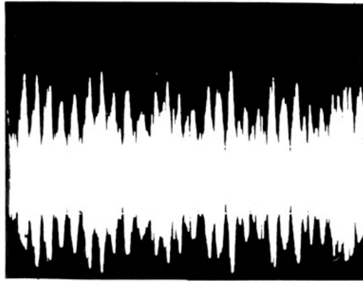
Fig. 9. Amplitude fluctuations of a 2-kHz tone recorded 60 m from a speaker in a deciduous forest. Total duration, 1 sec. (After Richards and Wiley, 1980.)
