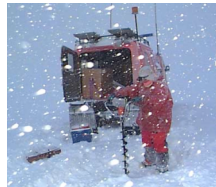
Scientist cutting a hole in the sea-ice with a petrol-operated ice-drill Image: Fiona Scott
