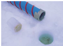
A Siple-corer and part of the resultant sea-ice core Image: Fiona Scott
